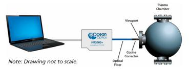
Figure 1: A modular spectrometer setup can be configured for plasma measurement in a vacuum chamber.
