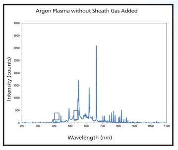
Figure 4: Argon plasma emission is measured in the vacuum chamber before the addition of sheath gas.
