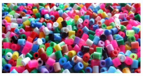
Polymers used in plastics have unique NIR spectral fingerprints that can be used for sorting and quality assurance throughout the life of the material. NIR spectroscopy can be used to sort and identify polymer resins prior to extrusion and later for rapid sorting of the product at recycling facilities. In this application note, the use of NIR spectroscopy for distinguishing colored plastic resins is described.
