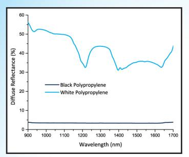
Figure 3: NIR-based sorting methods are not as effective with darker color samples, which absorb more of the NIR light.
