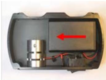
2. Insert batteries in the battery case as shown below.
