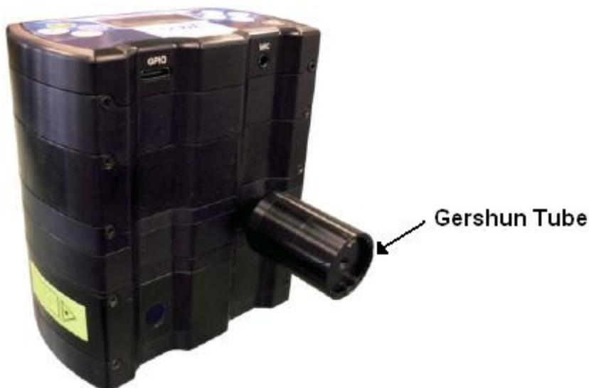
**Jaz Stack Spectrometer Module with Gershun Tube Attached**
