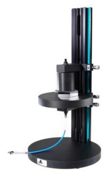
The Stage-RTL-T consists of a variable rail attached to a base plate, with three devices that attach to the rail with a thumbscrew. From bottom to top, these devices are a fiber holder with UV-VIS collimating lens; a sample holder for reflection or transmission; and a light trap to mitigate the effects of back reflection and ambient light. (Remove the light trap to access a second collimating lens.)
